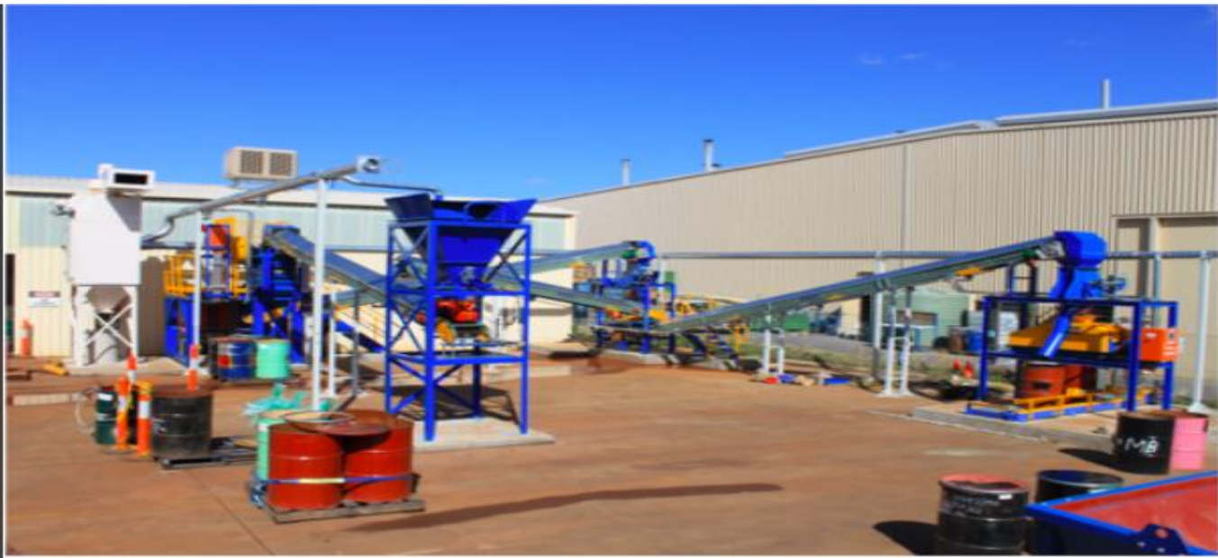
(Figure 1: Communitation circuit of the SGS test plant. It is anticipated that 3-4 5-tonne bulk samples can be processed per week by this facility. Bulk sample test work will be overseen by the existing scrutineering regime ensuring sample integrity in a certified laboratory environment.)
